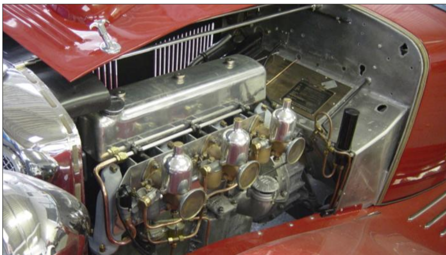
A general under-bonnet view of the author's SA 20. The vertical black tube on the right of the bulkhead is the fuel reservoir to keep a head of fuel in the float chambers. When new, the Speed Twenty was intended to promote quality with its well-finished engine parts and plated pipes under-bonnet. Following the successes of the Twelve-Fifty and Silver Eagle it had a lot to live up to. This engine is fitted with a later Silver Crest valve cover.
