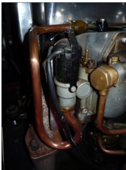
A close-up of the S.U. electric choke installation. As a non-original feature, it installed as discreetly as possible. With the adjustable jetting and air inlet, a fast idle on choke is useful. It does not require the mixture diffusion tube in the balance pipe as specified in the mid-period choke system.
